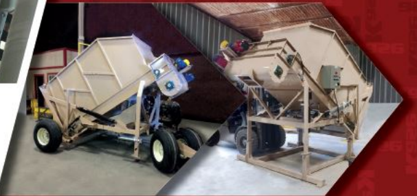
Left: Gobbler with custom hydraulic operated pneumatic tires > Right: 20' leg extension base for Gobbler
